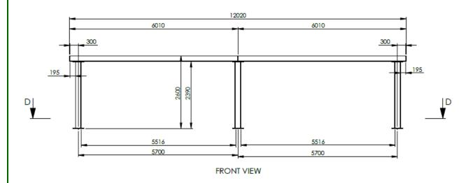
Legs and rails are made out of 200 UC.
